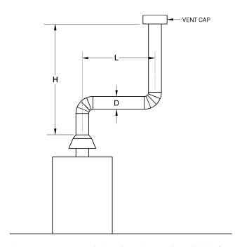
Asbestos cement Type B or single-wall metal vent serving a single draft-hood-equipped appliance [see Table C504.2(5)].
