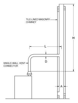
Table C504.2(4) is used when sizing a single-wall vent connector attached to a tile-lined masonry chimney.
