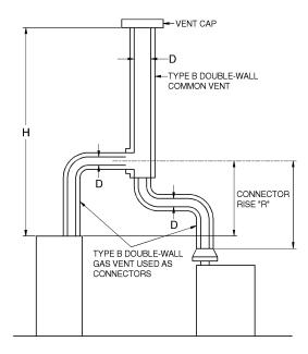
Table C504.3(1) is used when sizing Type B double-wall vent connectors attached to a Type B double-wall common vent.
