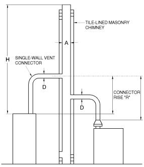
Table C504.3(4) is used when sizing single-wall metal vent connectors attached to a tile-lined masonry chimney.
