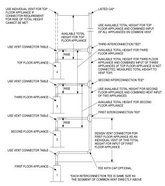
Principles of design of multistory vents using vent connector and common vent design tables (see Sections C504.3.11 through C504.3.17).
