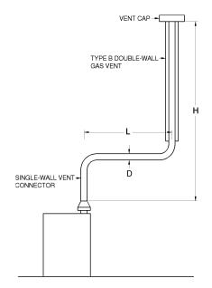
For SI: 1 foot = 304.8 mm, 1 British thermal unit per hour = 0.2931 W. Table C504.2(2) is used when sizing a single-wall metal vent connector attached to a Type B double-wall gas vent.
